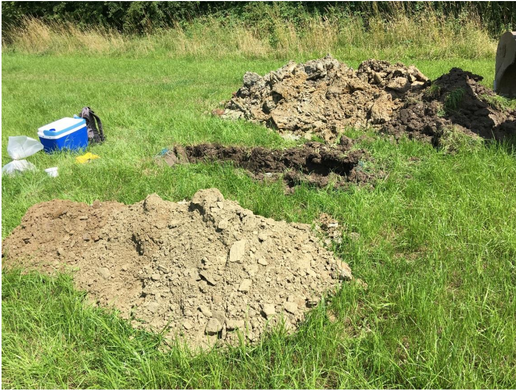
Spoil heap of TP07 showing siltstone of the Retford Member encountered at base
